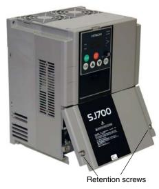
Notice the large power terminals at the bottom of the wiring area. The rubber grommets below the power terminals are for wire entry/exit to the power source and motor. Never operate the inverter with the front panel removed.
