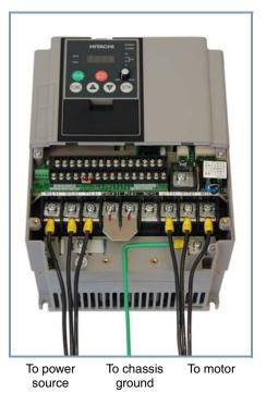
Use the same wire gauge on the motor and chassis ground wiring as you used on the power input wiring in the previous step. After completing the wiring:
