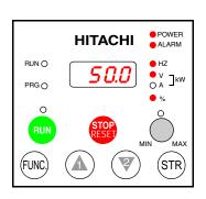
For the powerup test, monitor the motor speed indirectly by viewing the inverter's output frequency. The *output frequency* must not be confused with *base frequency* (50/60 Hz) of the motor, or the *carrier frequency* (switching frequency of the inverter, in the kHz range). The monitoring functions are in the "D" list, located near the top left of the diagram in the <u>"Keypad Navigational Map" on page 2–31</u>.
