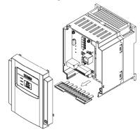
Screw for fixing the front cover is located at right-bottom side
