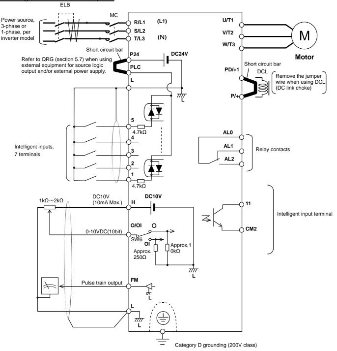
Note 1) Above shows an example of voltage (O) input. Changeover of SW6 must be done in case of current (OI) input. (Refer to page 9).
