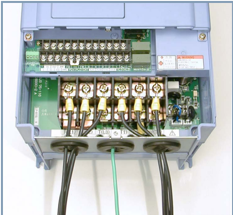
To Power Source To Chassis Ground To Motor
