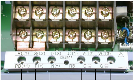
Retention screws locations for capacitor bank
